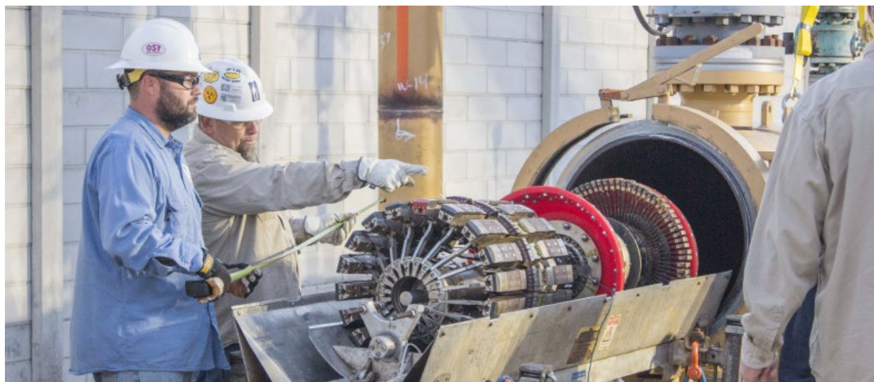
A "Smart Pig" is a machine that uses highly sophisticated sensors to provide information on how a natural gas pipe is performing.
