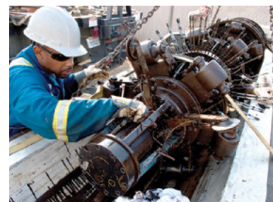
A natural gas pipeline inspection using a robotic smart "pig." Pipeline inspections improve safety and reduce fugitive emissions.
